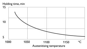
Note: Holding time = time at austenitising temperature after the tool is fully heated through.
