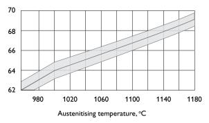
Hardness for different austenitising temperatures after tempering 3 times for one hour at  $560^{\circ}C \pm 1$  HRC.
