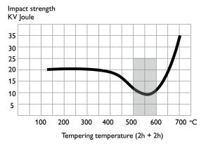
Tempering within the range  $500-600^{\circ}$ C is normally not recommended due to the reduction in toughness properties.
